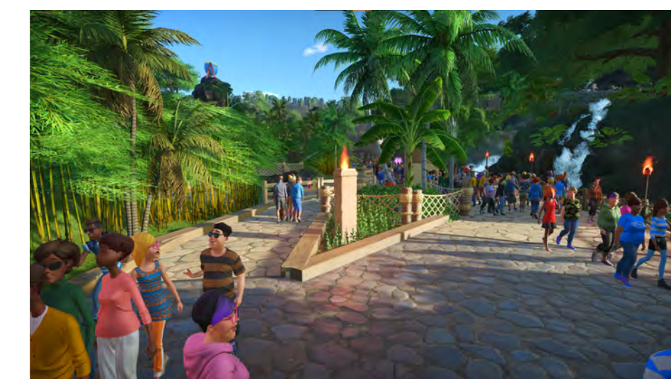
Wider pathways allow for guest distancing. All paths adhere to a grade of 5% or less to accommodate guests using mobility devices.
